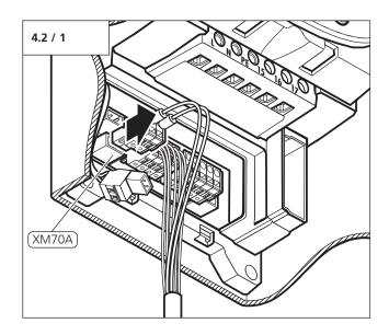
• Pull out the motor plug from the connection (XM70A).
