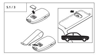
Visor clip, for attaching the hand transmitter to a visor in a car.
