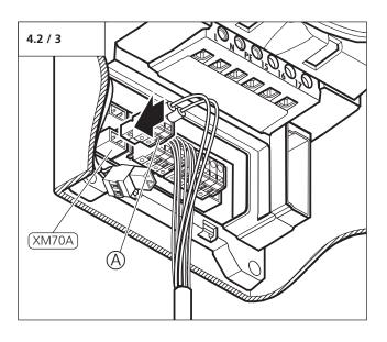
• Insert the motor plug (A) in the connection (XM70A).
