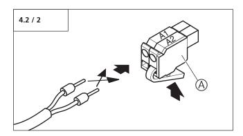
• Switch the positions of the leads in the motor plug (A).
