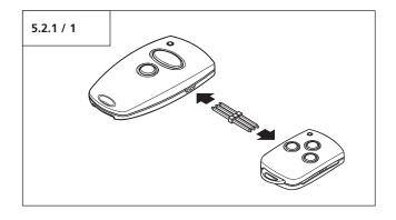
• Connect both transmitters with the enclosed transmission plug.
