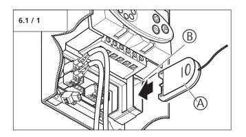
• Insert the modular antenna (A) into the antenna socket (B) in the controls.
